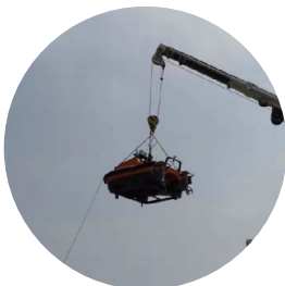
Designated Lifting system for Easy Launch & Recovery
